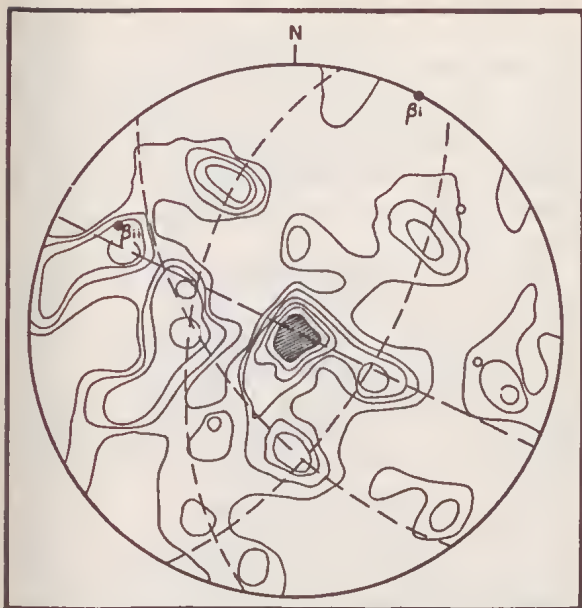
FIG. 11—Poles to foliation in gneiss at Mt. Beauty. Equal area projection, 224 poles. Contours 1, 2, 3, 5, 10, 15%.
